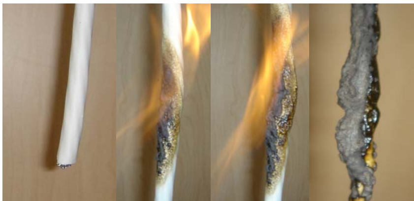
Fig 2: The intumescent char forming procedure of PE with JLS-PNP1C
